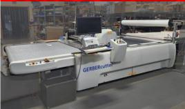
Gerber Model GTxL Automated Fabric Cutter
